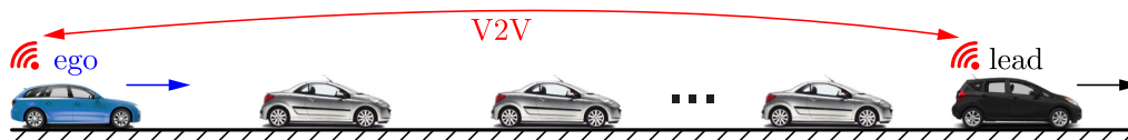
Figure 1: Connected vehicles traveling on the highway where an ego vehicle intends to predict its future motion based on a lead vehicle's past data.
